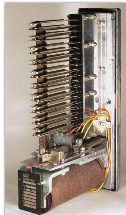
Figure 5: JRK relay type N
