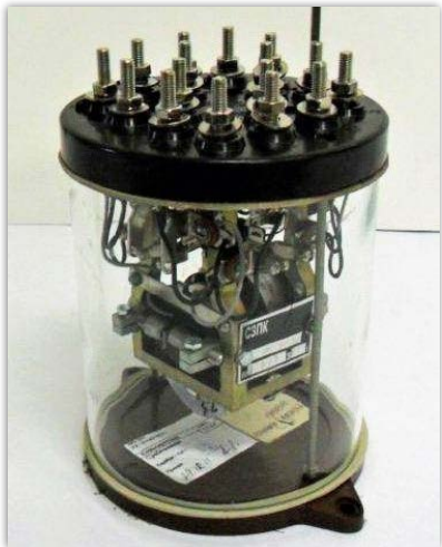
Figure 30: Shelf relay (Russian design)
