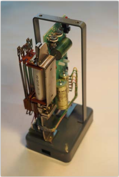
Figure 39: Delay unit type II WSSB with 'elementary relay' (relay not shown in fitting position)
